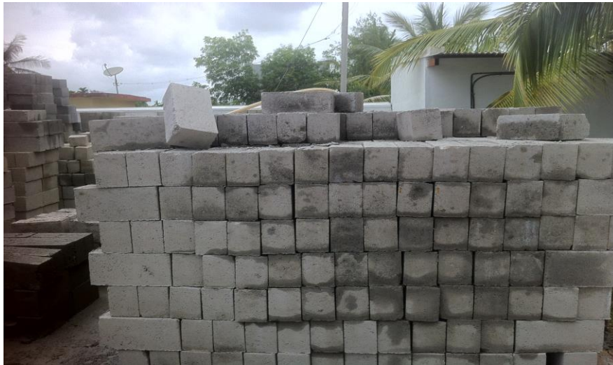
Bricks made from Fly ash – good acoustic & Thermal insulation properties
